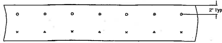
Stagger Pattern Plan and Elevation (Proposed Strip Floor) x ● ○ = Nail Row Designations
